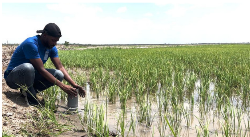
Dr. Abdul-Razak Saeed of UNDP demonstrating the installation of piezometer on a rice field
